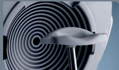
Placido disk - Measurement of corneal curvature radius
