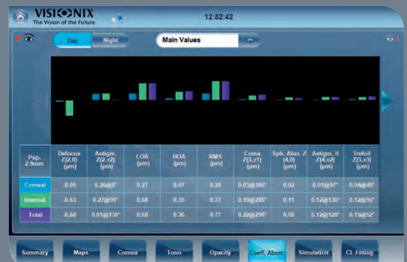
Analysis of aberrations with Zernike coefficients
